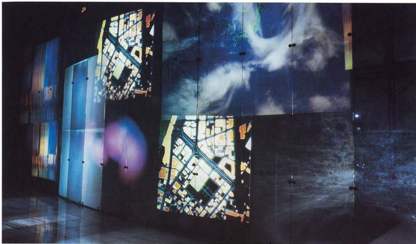
Dreams: A semi-transparent polycarbonete screen and luminous, semi-transparent acrylic and glass floor carry images from liquid crystal projectors.
