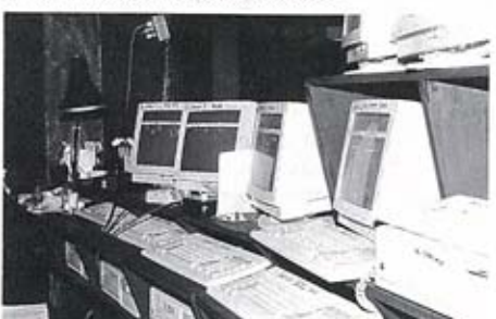
Control is provided by six Genesis computers with the operator's 'go' button just visible centre.
